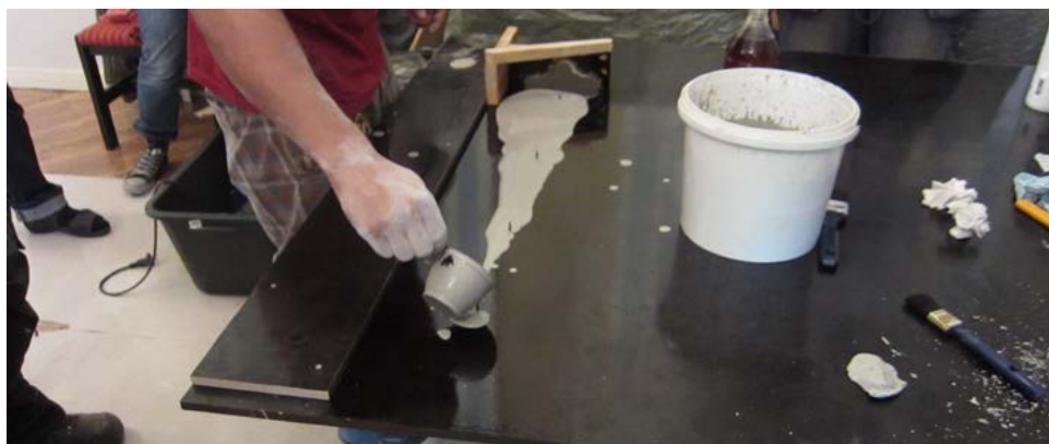
Figure 2.29. Plaster was mixed using a whisk and then poured on the table. The moulding sledge was pushed with metal side first to shape the plaster. Photograph by Meelike Naris.
