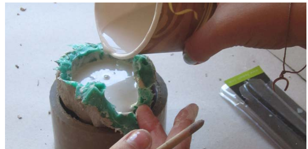
Figure 2.15. The silicone was stiffened with a crust of gypsum before it was taken off the model. Here a new head is in the making. Photograph by Sandra Heinström.
